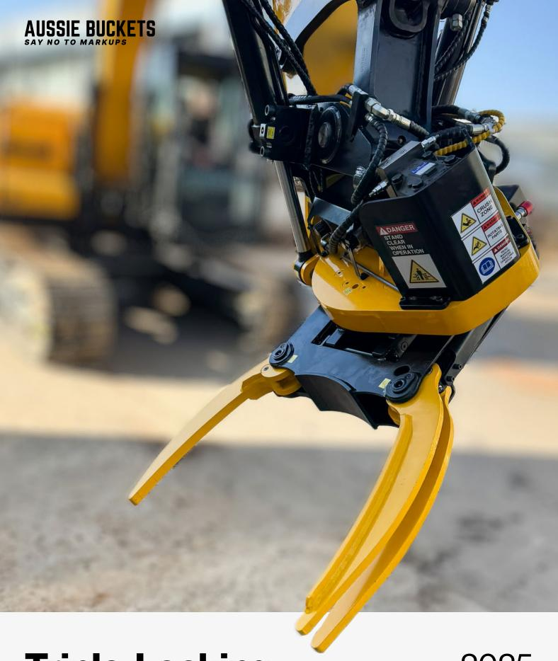
Triple-Locking Tilt Rotator
